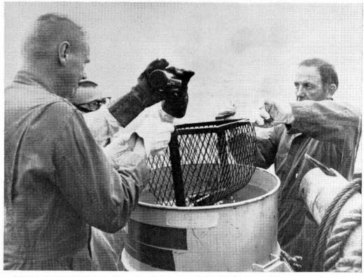
SAFELY RECOVERED from the ocean floor, two SNAP 19 fuel capsules are examined by (I to r) Bob Luikens (9521), Bill Gaines (3312) and John Adams (AEC/ALO) prior to shipment in a special container to Mound Laboratories. The two capsules, valued at \$700,000, survived rocket launch abort and almost six months under the sea in good shape. The cases around the plutonium 238 were undamaged.
